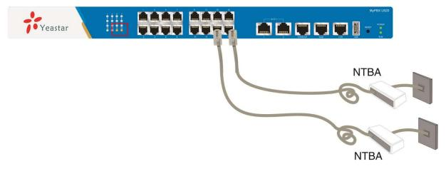
Figure 3-6 Connection of BRI ports and Status LED
