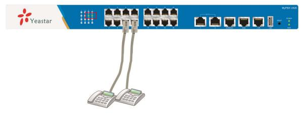
Figure 3-7 Connection of FXS ports and Status LED
