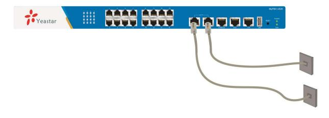
Figure 3-2 Connection of E1/T1 port
