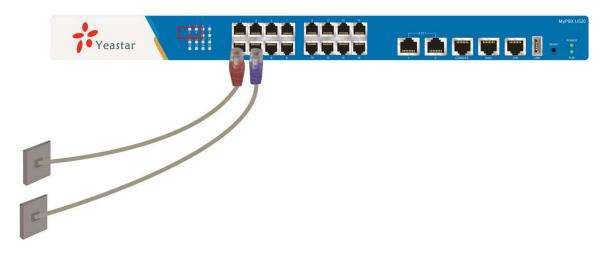
Figure 3-3 Connection of FXO ports and status LED
