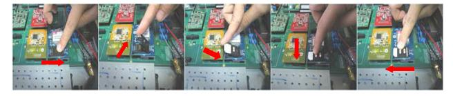
Figure 3-4 Inserting the SIM Card
